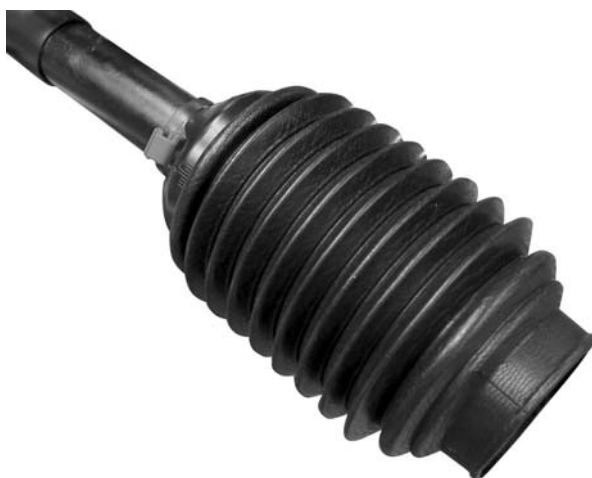
Figure 3.3 : Protection de la transmission
